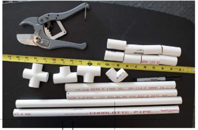
Figure 19- PVC connectors and pipes for measurements
